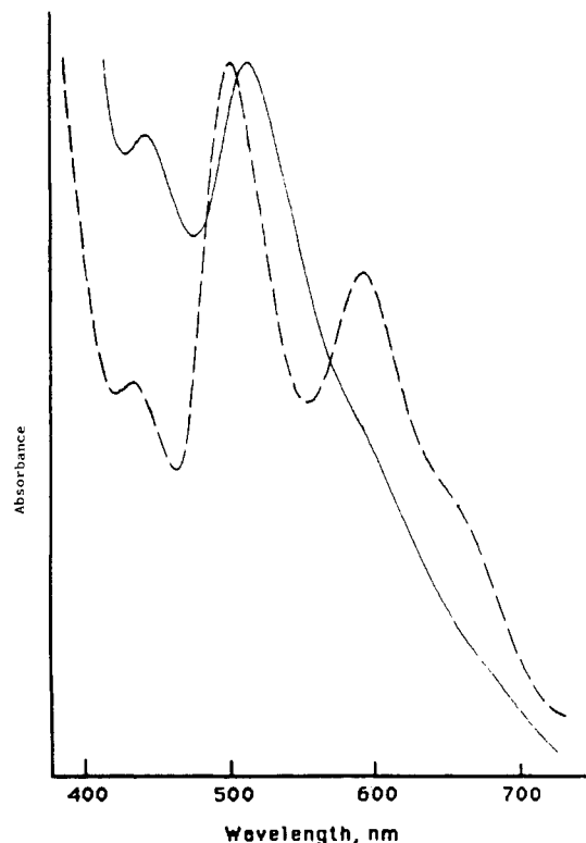
Figure 2. Electronic spectra of \text{Cp}_2\text{TiI}_2 (---) and \text{Cp}^*_2\text{TiI}_2 (—) in benzene solution. The absorbance scale is relative; see Table III for \epsilon values.
